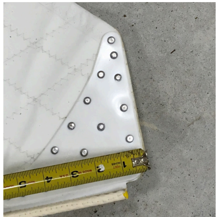
Picture 4: Measurement not to exceed as taken from headboard.
